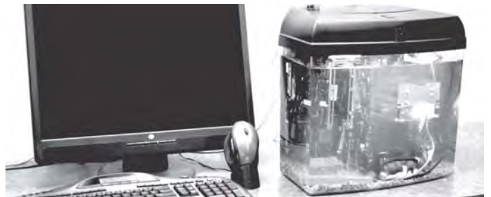
Puget Systems Mineral Oil Cooled Computer Case
